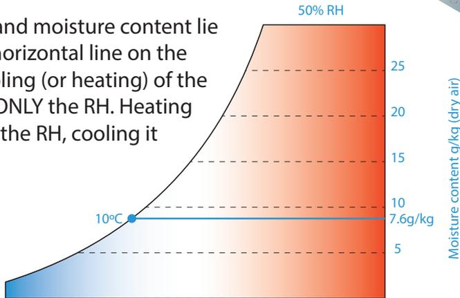
If a dewpoint is measured, a g/kg figure can be determined directly from the chart. The line on the chart between dewpoint and g/kg is direct and does not change. If, for example, the temperature rises and falls, neither the dewpoint nor the g/kg alters.
